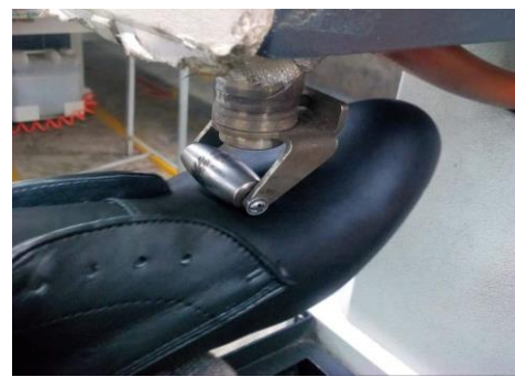
Figure: Ironing with hot air blow
