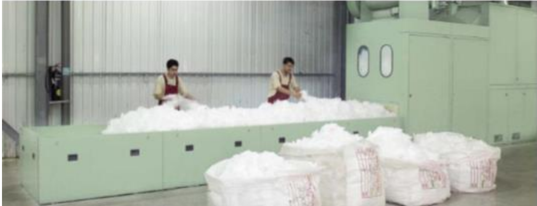
Fig: Small lots of fibers are feeding manually
